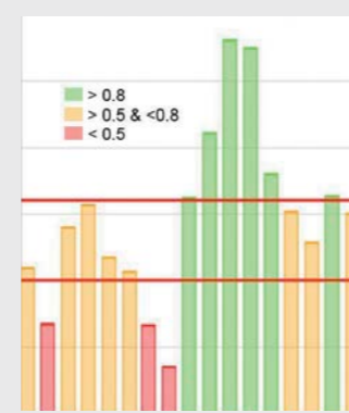
Fig. 2 Solar DHW production performance monthly ratio from 09/2012 to 01/2014 on a social housing building - GOSPELS project
