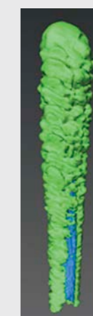
Fig. 1 3D reconstructed structure of the fresh Pt 3 Ni 7 NSTF obtained using electron tomography
