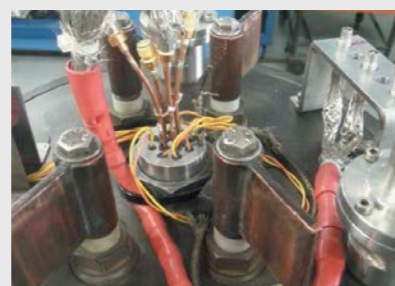
Fig. 1 Plug with feedthroughs for capacitive sensors and TCs
