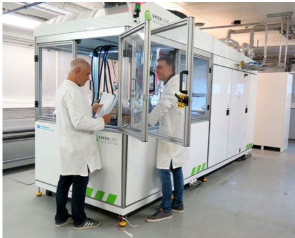
The PEMFC platform ramps up with the acquisition of a 100kW test bench.
